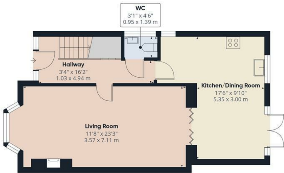
Ground Floor Building 1
